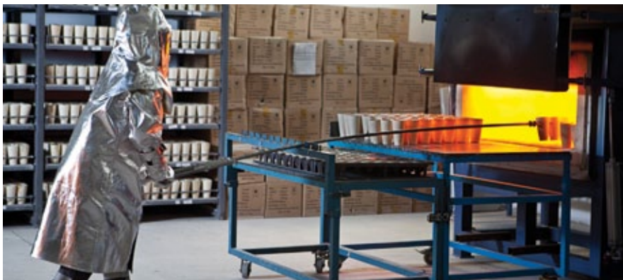
Multi pouring of 84 geochem sample set fusion for gold determination by fire assay. Photo courtesy of SGS.
