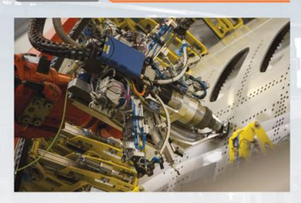
Within the Aerospace Field, Bisiach&Carrù is specialised in drilling and riveting automation with the Tauro system.
