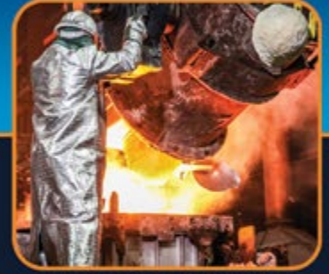
Description of picture: Feeding an automatic pouring station
