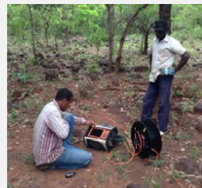
Geophysical technician at IP measuring station for 800m electrode spread
