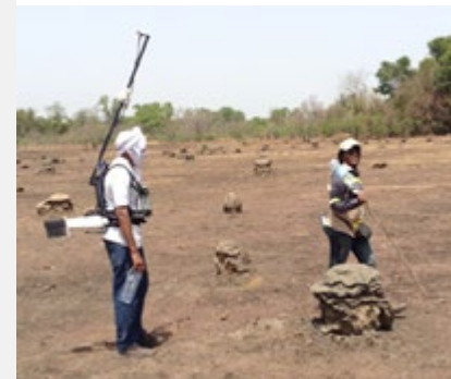
Geophysical Technician and geologist on a combined VLF & ground magnetic survey in northern Cote d'Ivoire
