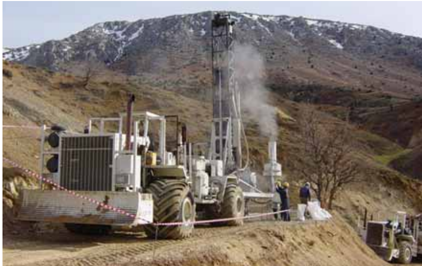
A reverse circulation drilling rig at Anatolia Minerals' Çöpler mine.
