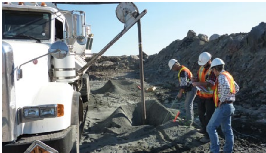
Dyno Nobel's Titan emulsion being loaded at Cliffs' Bloom Lake iron mine. (Photo courtesy of Dyno Nobel)
