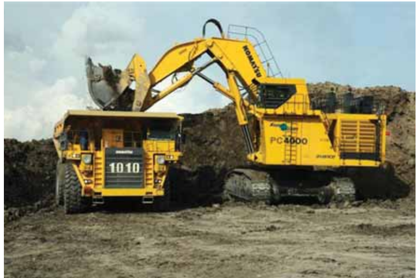
Overburden stripping at Tutupan - PT Adaro.
