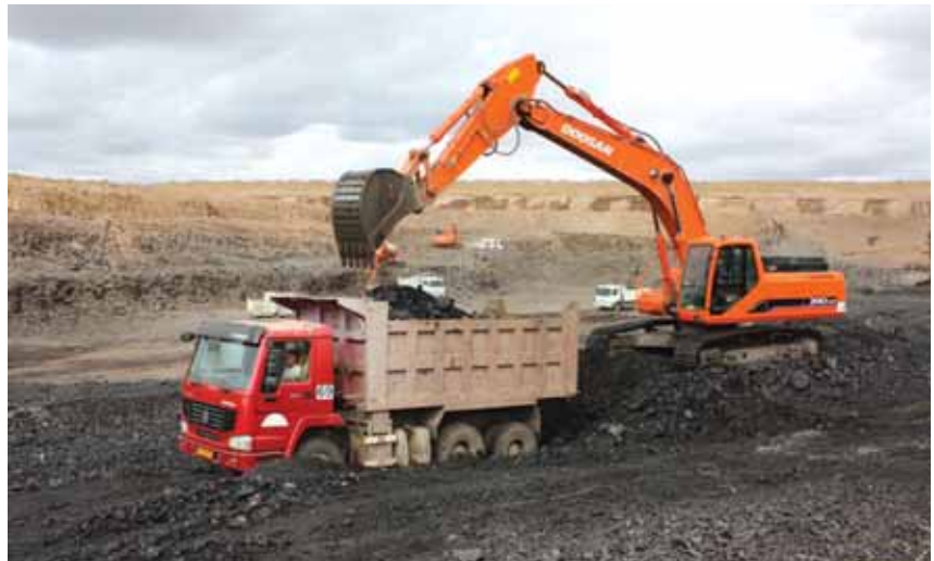
Saryarka—loading coal from mine into haul truck.
