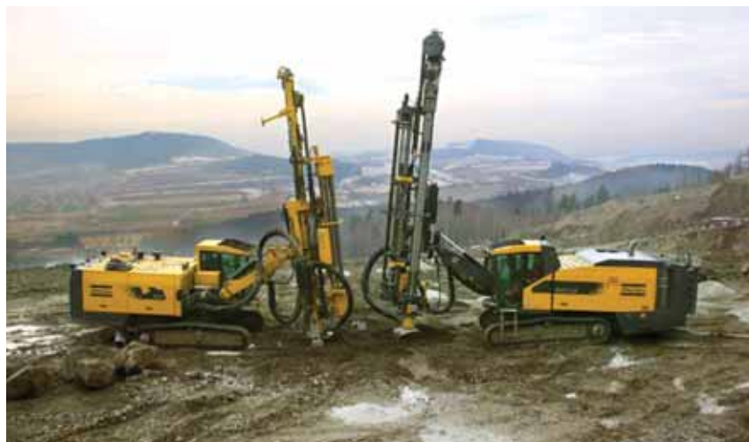
Blasthole drilling in Kazakhstan with Atlas Copco ROC L6 drills. (Photo courtesy of Atlas Copco Kazakhstan)
