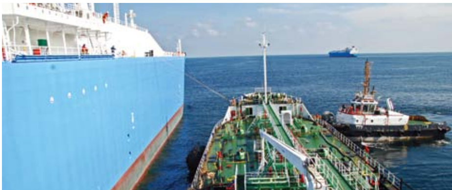
Floating Storage Receiving Unit for LNG Pertamina
