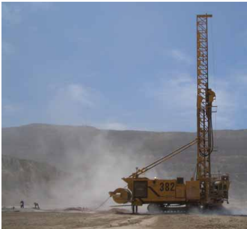
Electric blast hole drill, drilling at 11 of diameter at the same mining site (Chuquicamata Codelco) since 2006.
