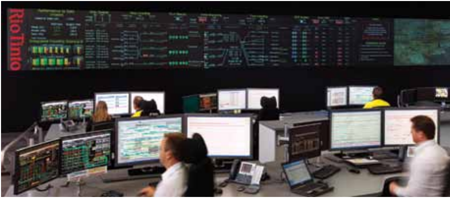
Rio Tinto's "mine of the future". The interior of the Operations Centre in Perth from where trucks are operated remotely. (Photograph courtesy of Rio Tinto).
