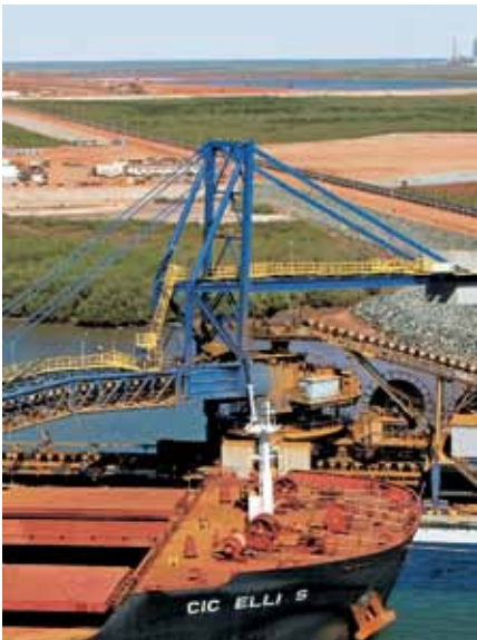
Fortescue Metals Group's Pilbara Iron Ore and Infrastructure Project - Shiploader at Anderson Point Berth, one of many projects that WorleyParsons contributed to in Australia.
