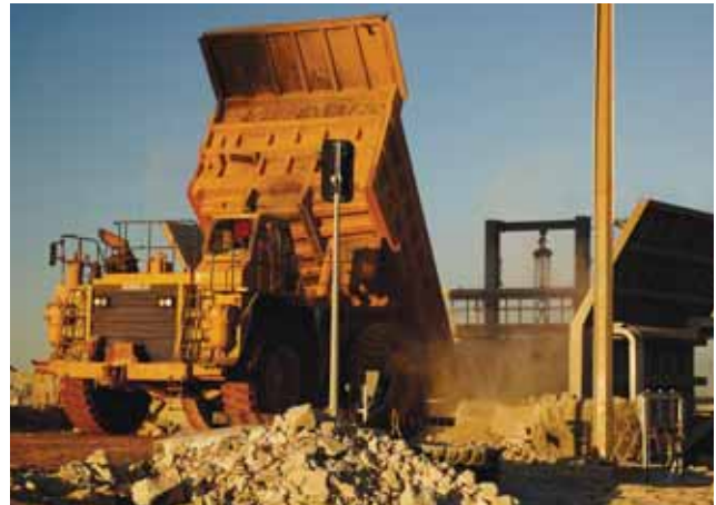
Gold-copper ore at Telfer being dumped into primary crusher.
