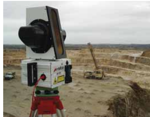
Maptek's new I-SiTE product is capable of combining detailed laser imaging with real panoramic photography.
