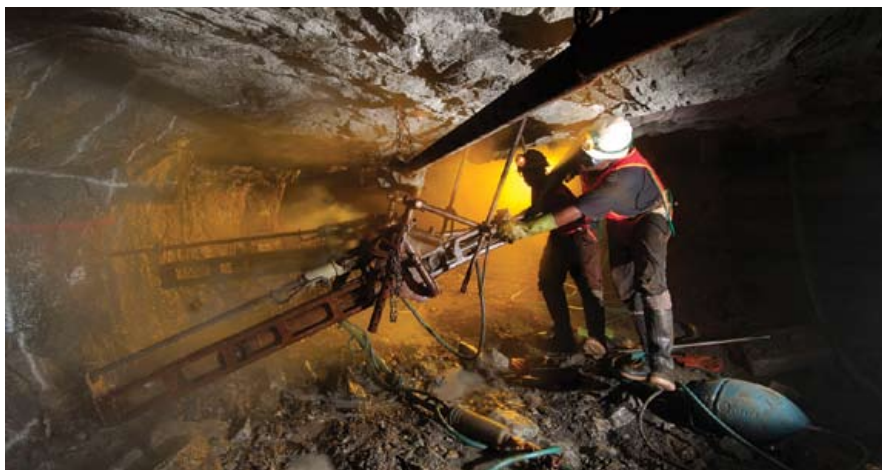
Platinum miners operate jackleg drills in a low-profile reef formation. (Photo courtesy of Implats)
