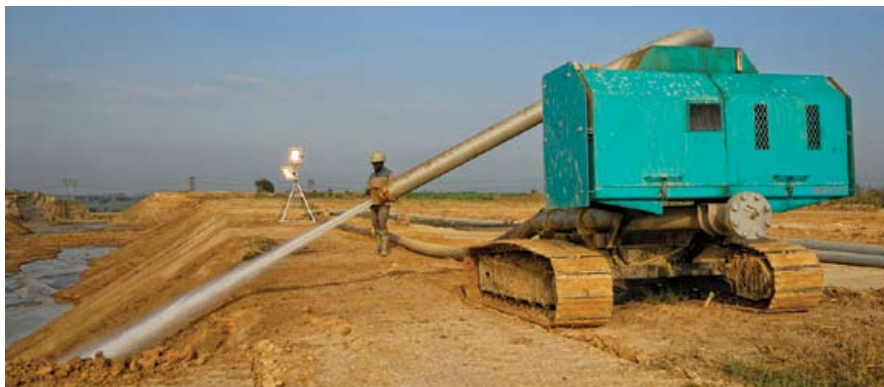
Hydraulic re-mining with a Fraser Alexander Track Gun. (Photo courtesy of Fraser Alexander)
