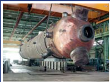
FESSENHEIM, France, feedwater heater for CNPE
