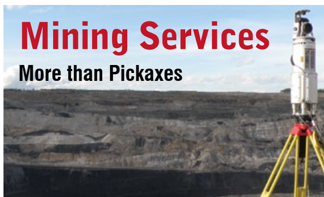
Terrestrial laser scanning for mine reconciliation survey. Photo courtesy of McElhanney.
