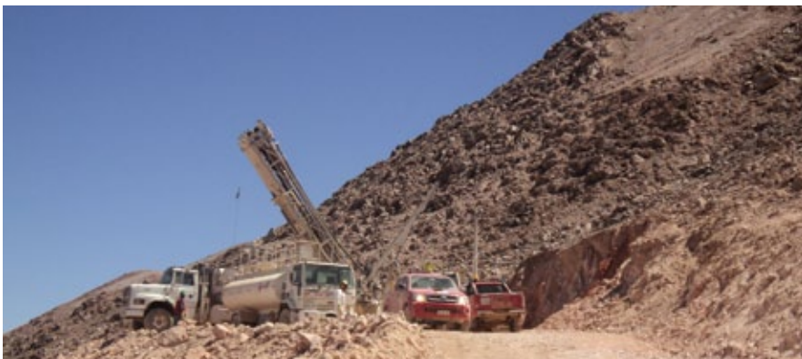
RC drilling at the Cerro Buenos Aires exploration target, Pampa Buenos Aires project. (Photo courtesy of Iron Creek).
