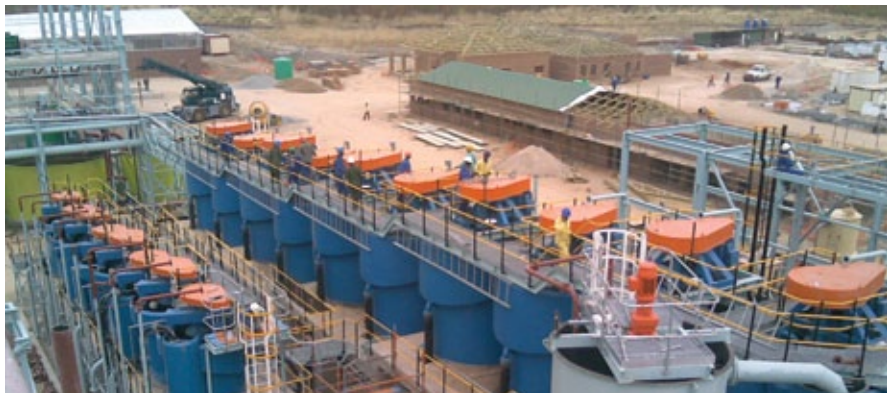
Delkor designs and manufactures mineral processing equipment, such as floatation cells. (Photo courtesy of Delkor).
