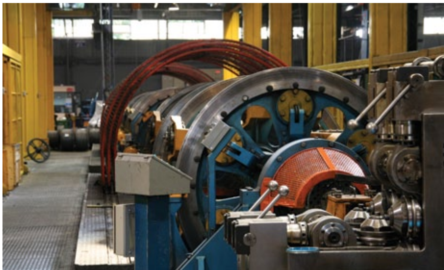
Planetary strander for production of shovel rope strands. (Photo courtesy of Prodinsa).
