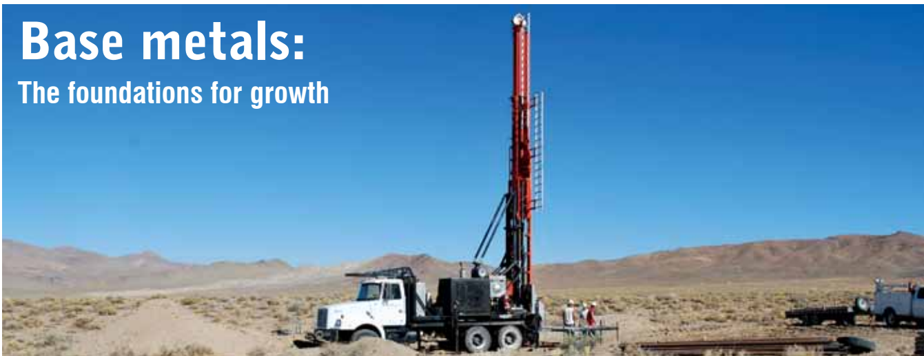
Entrée Gold currently has an extensive drill program under way at its properties in Yerington, Nevada. Pictured above is a diamond drill on the Ann Mason property.
