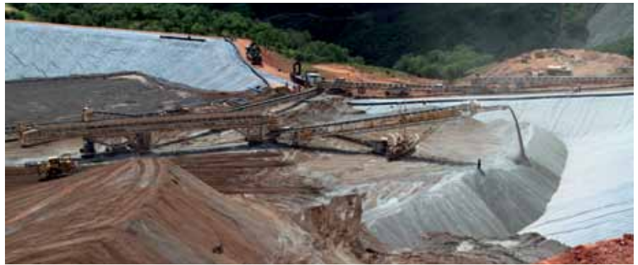
Loading ore to Phase 2 Leach Pad at Minefinders' Dolores mine.
