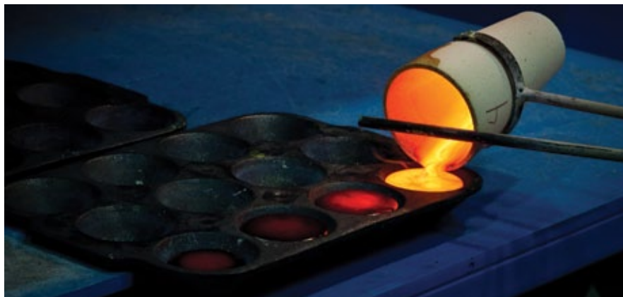
Pouring of a molten fire assay product. Photo courtesy of Met-Solve Laboratories.
