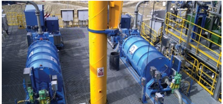
The Antapaccay M3000HF IsaMills, the first operating in South America. Photo courtesy of Xstrata Tech.
