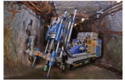
SBM 400 SR for slot raises at Milpo mine, Peru
