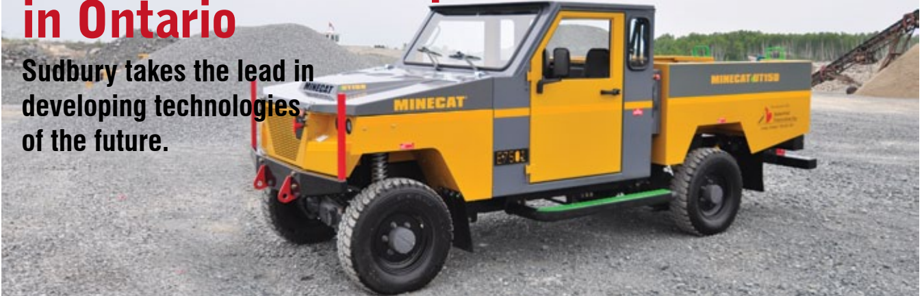
The Minecat UT150-eMV is the first electric utility vehicle approved for 20% ramp travel. Photo courtesy of Industrial Fabrication.
