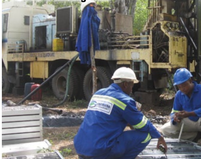
Geological technical assistants inspecting coal cores during a drilling stand-by at Moatize coal field. Photo courtesy of Gondwana.
