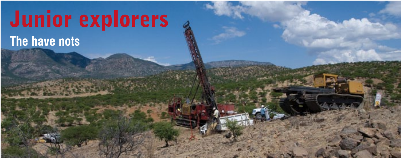
Diamond drill rig at the Coneto silver-gold project, Coneto de Comonfort, Durango State, Mexico. Photo courtesy of Orex Minerals.
